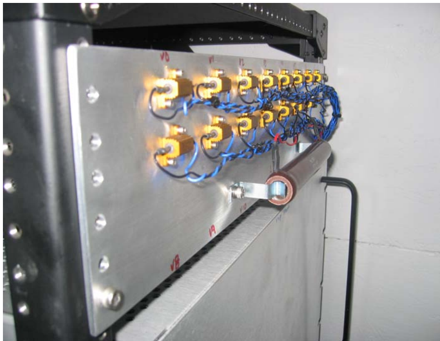
ARRO TEST DUMMY LOAD (TO SIMULATE 16 INSTRUMENTS DISSIPATING A TOTAL OF 50 WATTS)
