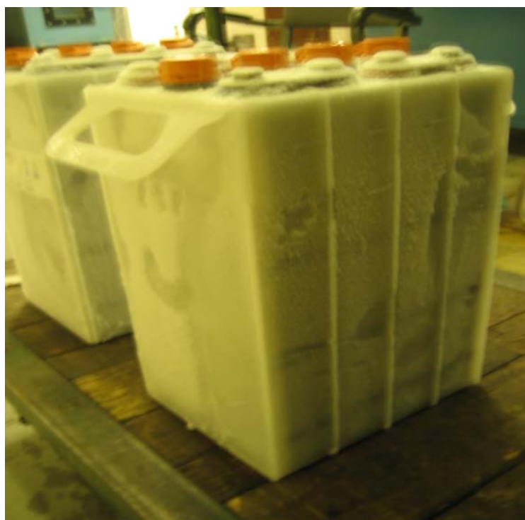
SUNICA PLUS BATTERIES: POST COLD SOAK TESTING
